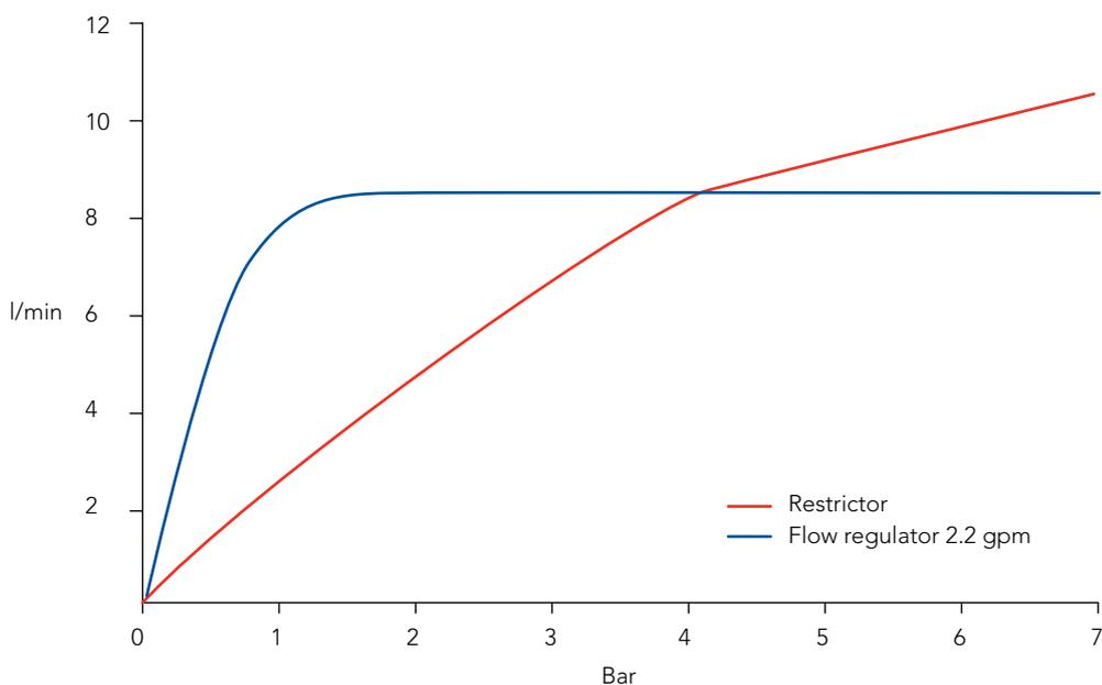
**Figure 10** Comparison of a conventional restrictor with a pressure-compensating flow limiter insert.
