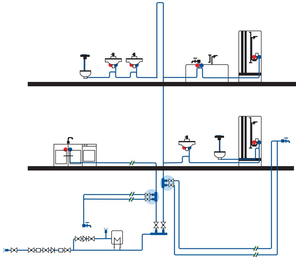
**Figure 20** Example of a water supply layout in dwelling with high use kitchen sink, showers and WC, but low use external taps. All terminal branches are kept as short as possible. The vertical loop on the upper floor is for a future extension of the water supply system.
